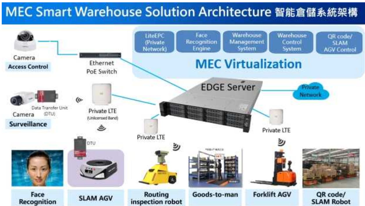
[그림 6 MEC Smart Warehouse Architecture, Foxconn ]
