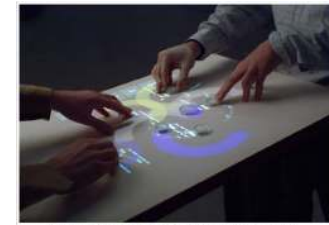
Figure 1: The Audiopad electronic music controller.
